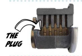
The plug surrounds the keyway, rotates freely within the housing, creating a rotational shear line. Consider this as the "bottom paper."
