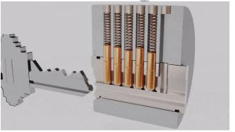
The springs have two jobs: forcing everything down into the plug and push the key pins against the key, which helps read the cuts of the key. Without springs, the pins could get stuck anywhere in the pin chamber.
