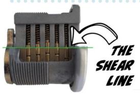
The shear line is where the plug and and hull casing meet. The goal of lockpicking is to manipulate the pins so that driver prins are above the shear line and key pins are still within the plug, allowing rotation and unlocking.
